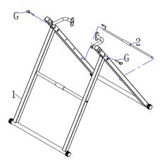
A.Open the front and rear supports holder (1) of the inversion machine, and insert the pull-ring pin (G) into the hole at the connection between the front and rear supports holder.
