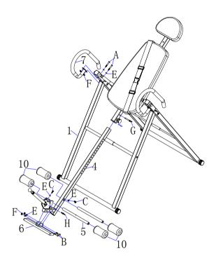
A. Insert the foam tube (5) into the large hole on the height adjustment frame (4), and fix it with screws (C) and flat washers (E). Put the foam (10) into the foam tube from both ends (5) on;
